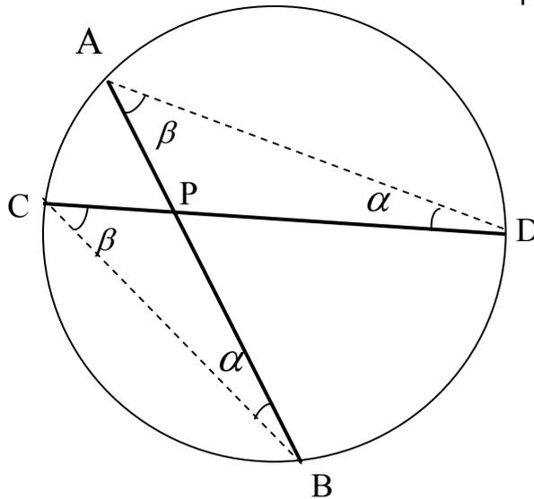
$\Delta APD \sim \Delta CPB$ :  $PA \times PB = PC \times PD$
